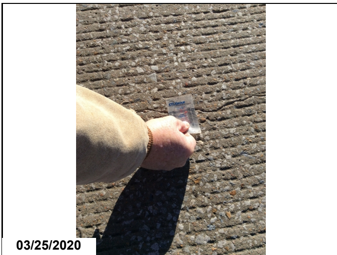
Moderate width deck cracking.
